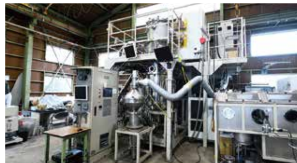
Equipment for manufacturing gas atomized powder, which is the material for metal 3D printers. The demand for this material has been increasing in recent years, and MAKABE GIKEN has been developing and manufacturing it for over 30 years.
